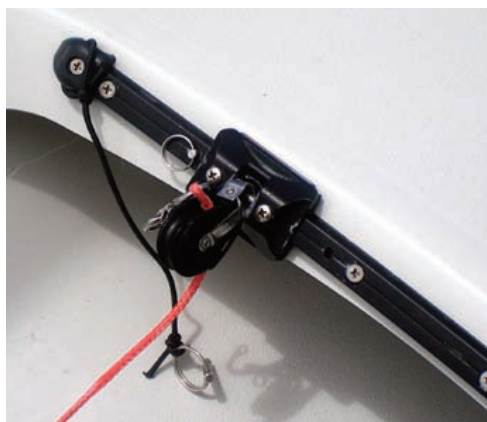
Jib car pin in outer position
